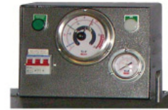
The Temperature Control Unit regulates the temperature range of the Flux.
